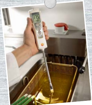
Checking the quality of the cooking oil in a deep-fryer
