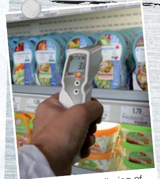
Fast and easy monitoring of products in refrigerated shelves
