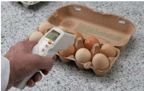
Fig. 5: Infrared measurement of surface temperature on foods
