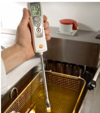
Fig. 12: Measurement of the TPM value in cooking oil with the testo 270
