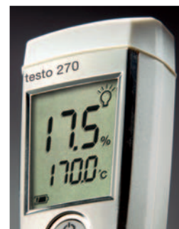
Figure 25: Visual and acoustic alarm if a given limit is exceeded
